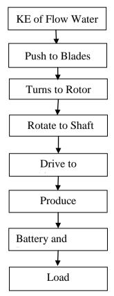
Figure 1 The working procedure of flow turbine
