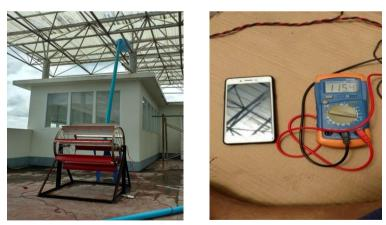
Figure 8 Test run of flow turbine by 2-inch pipe and 10 feet height.
