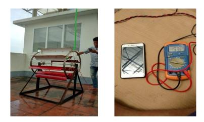
Figure 9 Test run of flow turbine by 1-inch pipe and 10 feet height
