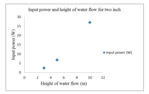
Figure 11 Input power depend on height of water flow with 2 inch pipe
