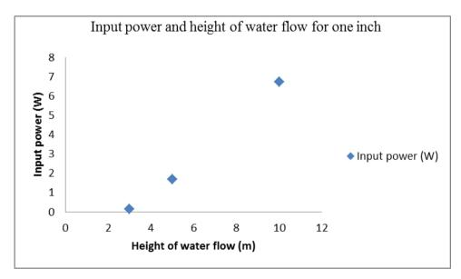
Figure 10 Input power depend on height of water flow with one-inch pipe
